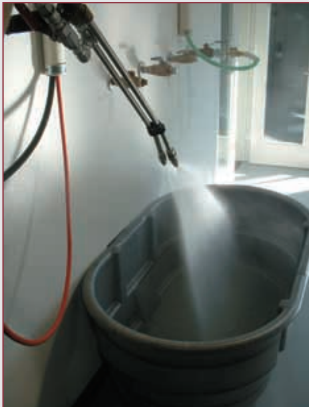
> The WhiteWater system simultaneously applies, in two parallel streams, low-pressure ozone-infused cold water and high-pressure cold water to dirty surfaces.
